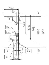
**Electric** Supply voltage: 400 V/3N ph/50/60 Hz Total Watts: 1.5 kW Water: Inlet water line size: 3/4" Incoming Cold/hot Water line 3/4" Drain line size:
